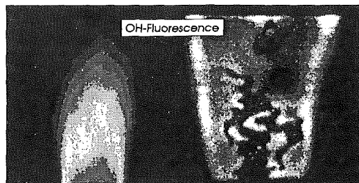
Fig. 21 Laser-induced fluorescence (right-hand side) and self-induced fluorescence (left-hand side) from a Bunsen flame
